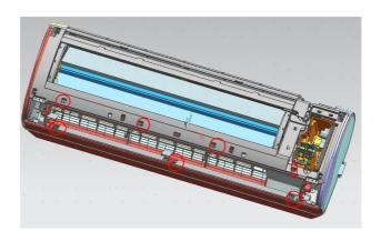
Release the marked hooks on the top side of unit and then pull the front grille out horizontally and remove it
