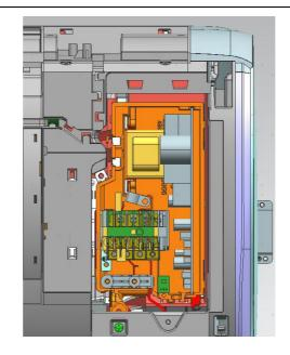
5 Lift up the three screw covers and then loosen the marked seven screws
