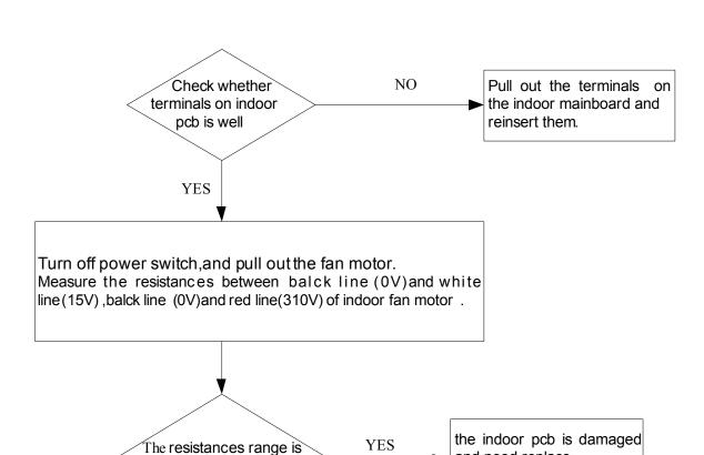
The indoor fan motor is damaged and need replace
