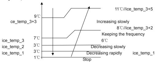
When Tpg\_indoor  $\langle$  ice\_temp\_1 $^{\circ}$ C, the frequency of the compressor decreases at the speed of 1HZ/1second.
