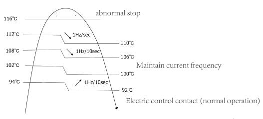
TTC>=116  $^{\circ}$ C lasts for 20 seconds. Overheating protection of air-blowing, compressor stops for more than 3 minutes
