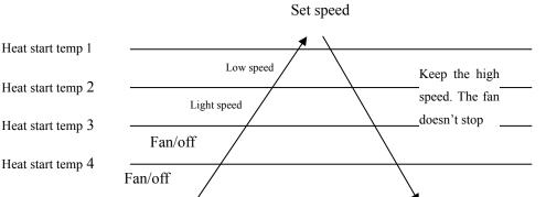
2. 4 minutes after the start up of the indoor fan, the light airflow and the low airflow will be turned to the set speed airflow.
