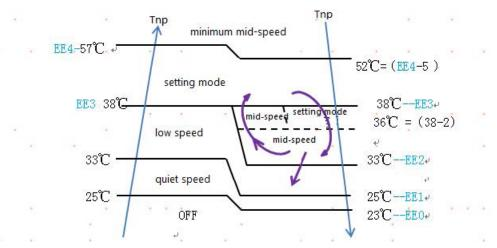
\* Residue heat sending. The indoor fan will send the residue heat at a low speed for 20 seconds. If other conditions are satisfied, when the compressor stops, the indoor system will operate at a light speed. The indoor fan will stop when the coil temperature (Tnp) is below the THHOT0 (EEO).
